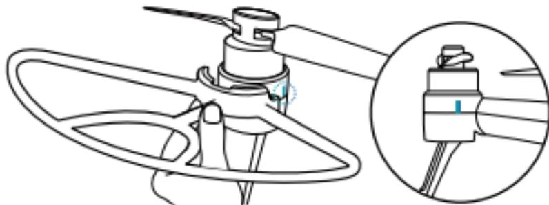
To remove the propeller protectors, unlock them from the engine arm from one side to another.
